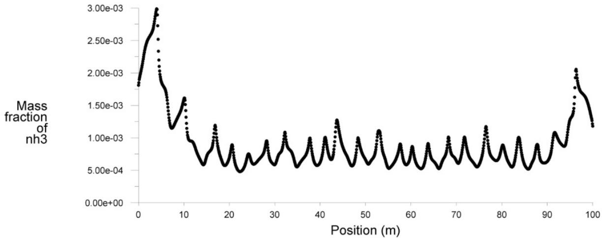
Fig. 3. Mass fraction of  $\text{NH}_3$  in case of transversal ventilation
