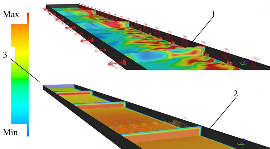
Fig. 4. Comparison of flow pattern for transversal and longitudinal ventilation: 1 – transversal ventilation:  $\text{min} = 0 \text{ m}\cdot\text{s}^{-1}$ ,  $\text{max} = 1.6 \text{ m}\cdot\text{s}^{-1}$ ; 2 – longitudinal ventilation:  $\text{min} = 2 \text{ m}\cdot\text{s}^{-1}$ ,  $\text{max} = 2.7 \text{ m}\cdot\text{s}^{-1}$ ; 3 – level of velocity
