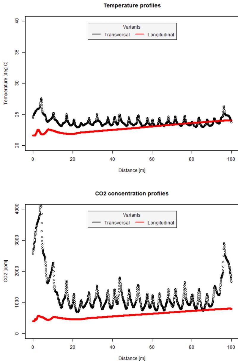
Fig. 5. Comparison of temperature and CO<sub>2</sub> mass fraction in central axis of the stable at the height 0.5 m above the floor
